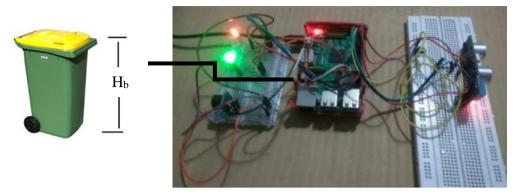
Fig. 5. IOT Module Integrated to the Smart Waste Bin
