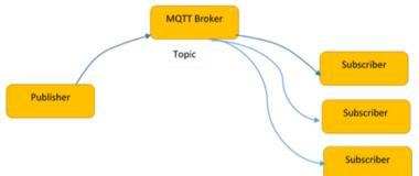
Fig. 2 MQTT Protocol Topic Transmission
